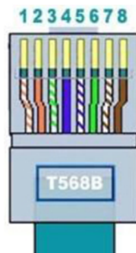
Wiring order (1-8) according to T568B standard: white-orange, orange, white-green, blue, white-blue, green, white-brown, brown
